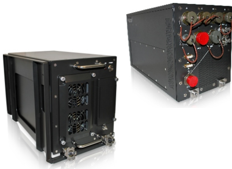
Trenton TMS6700 Military Computer Shown with one shoe-box backplane and one SBC
